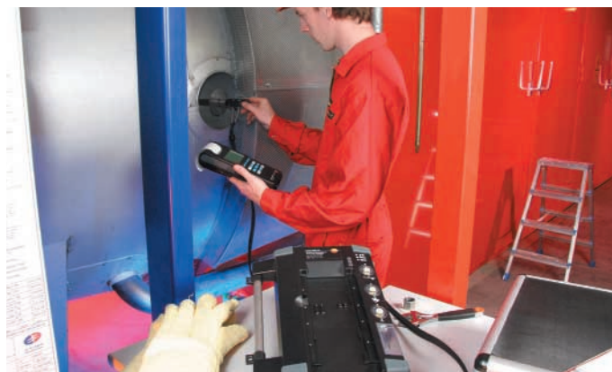
testo 350 XL: Portable measurements on turbines (O 2 , CO low , NO low , NO 2 )
