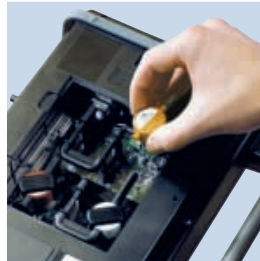
Fast-action and user-friendly measurement cell exchange by the user on site
