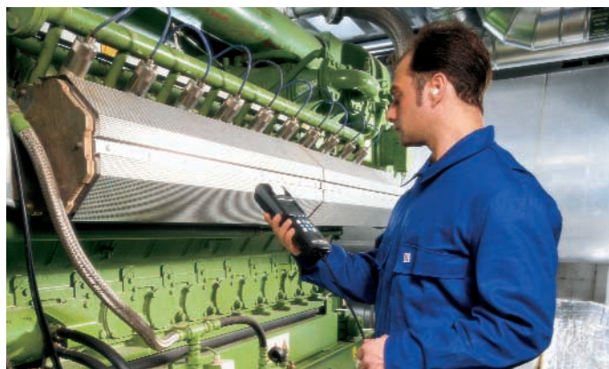
testo 350 XL: Portable measurements on motors (O 2 , CO, NO, NO 2 )
