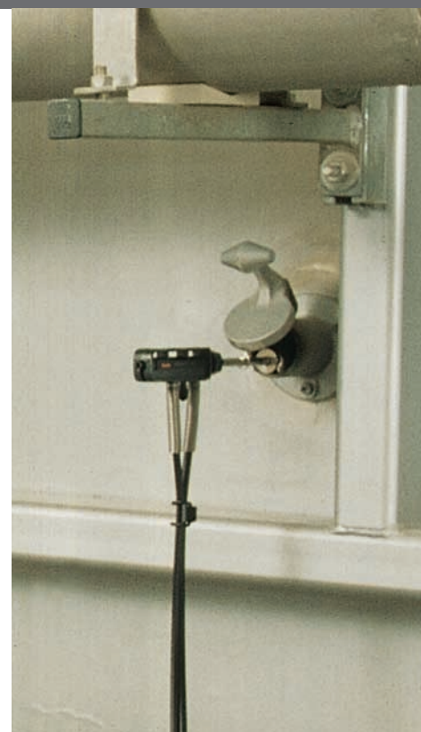
Standard gas sampling probes, available in lengths of 335 mm and 700 mm
