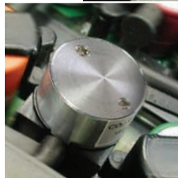
Infrared (NDIR) measurement module for direct CO 2 measurement
